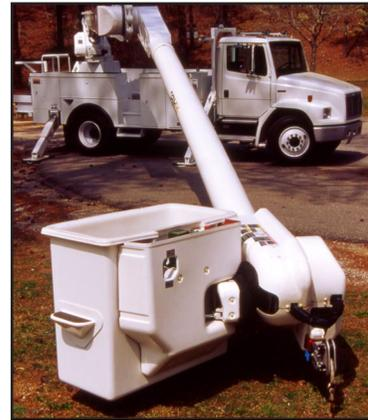
Compact boom tip design allows operator to get close to the work and maneuver in congested areas
